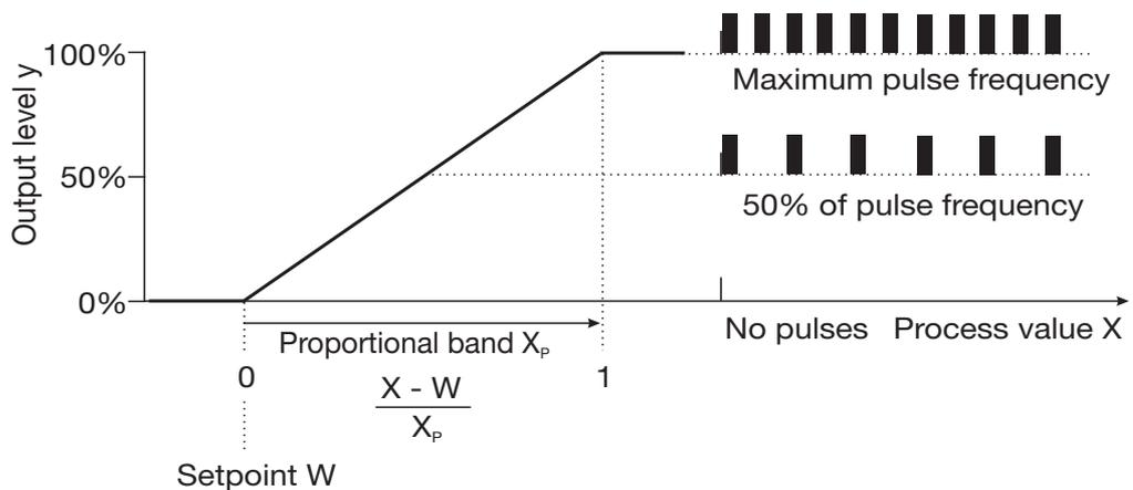
If actual value  $x$  exceeds setpoint  $W$ , the P controller will control in proportion to the control deviation. When the proportional band is exceeded, the controller operates with an output level of 100% (maximum switching frequency).
