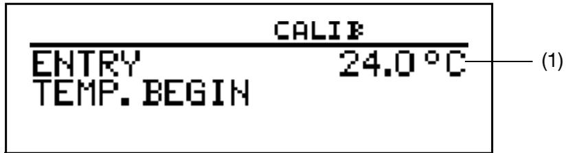
Enter the required start temperature (1) for the temp. coef. curve.
