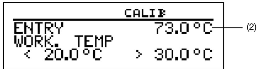
The LC display now shows the chosen working temperature (flashing) (2).
