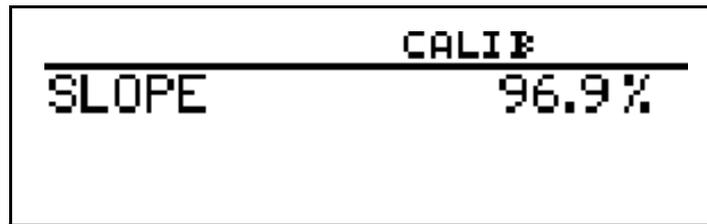
The slope determined by the device is displayed.
