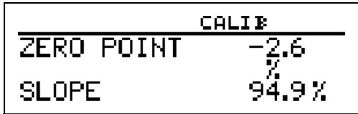
The LCD display shows the following calibration results:
