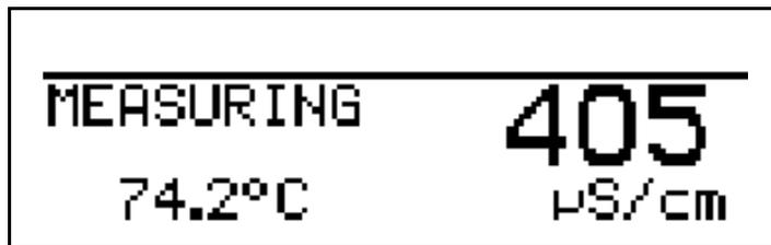
The transmitter is in "measuring mode" and displays the compensated conductivity of the solution.
