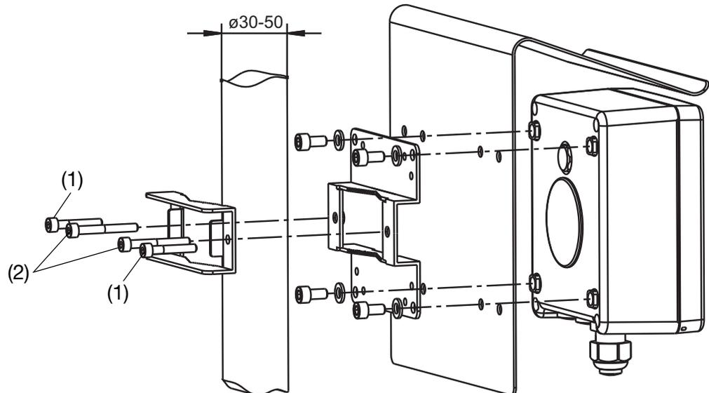
Screws (1) M5 x 30 for pipe diameters from 30 to 40 mm.
