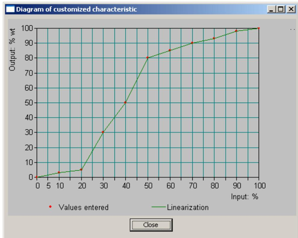
The optional setup program is used to enter the requisite value table.
