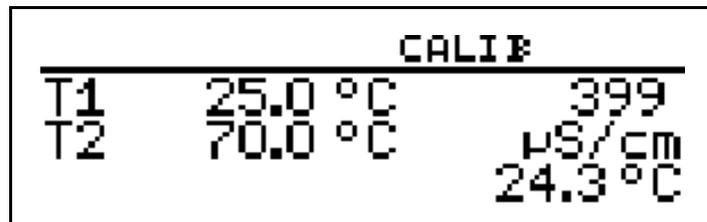
The conductivity (399 µS/cm) at the current temperature (24.3°C) now appears on the right of the LC display.
