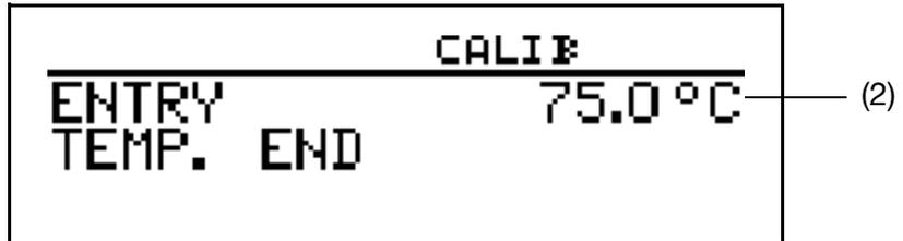
\* Enter the required end temperature (2) for the temp. coef. curve.
