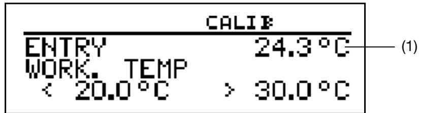
The displayed current sensor temperature flashes (1).
