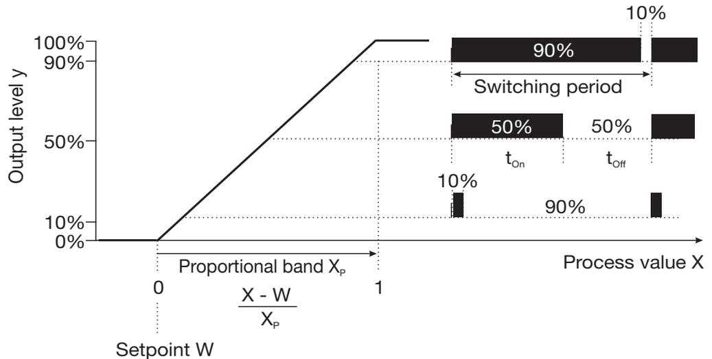
If actual value  $x$  exceeds setpoint  $W$ , the P controller will control in proportion to the control deviation. When the proportional band is exceeded, the controller operates with an output level of 100% (100% clock ratio).
