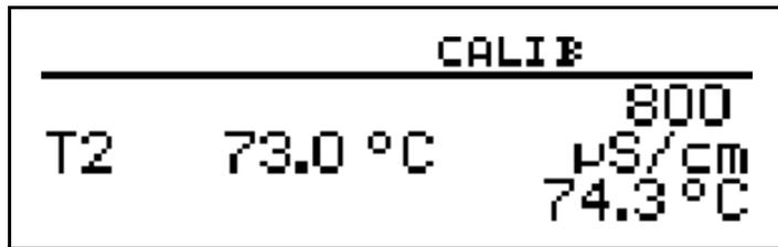
If the temperature of the medium exceeded T2 (73.0°C), the device determines the temperature coefficient.
