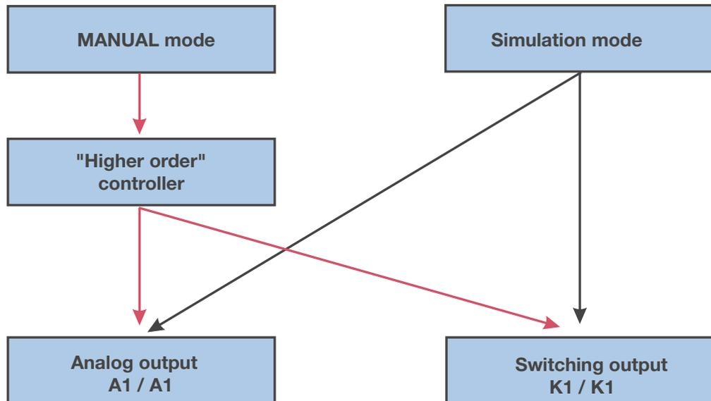
Simulation mode **directly** accesses switching outputs K1/2 or analog outputs 1/2. When simulation mode has been selected, MANUAL mode is **not** possible!
